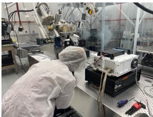
Theodolite measurements of PIG#2 collimated image in clean room
